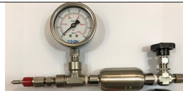
Inlet Gas Sampling with 50 ml bottle
