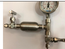
Outlet Gas Sampling bottle capacity 50 ml with Septa
